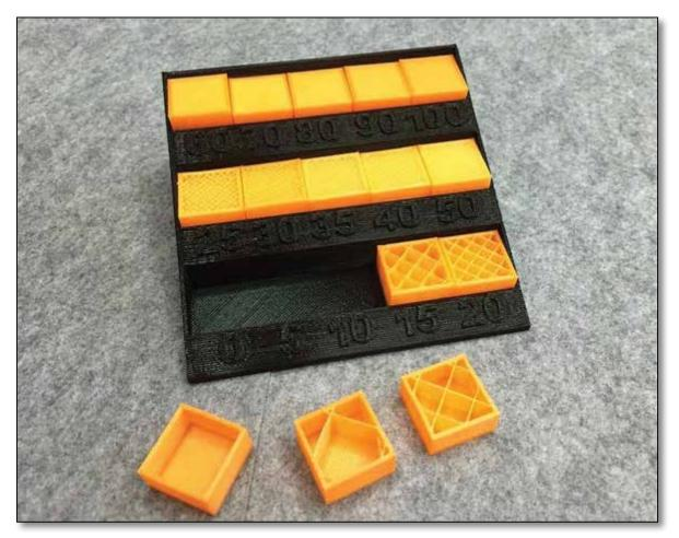
**Print-speed:** refers to the speed at which the print-head nozzle travels while it lays down clay. Optimal settings depend on the design, the nozzle size, the layer height and clay adhesion properties. The trade-off between high print-speed and lower quality is a personal one.
